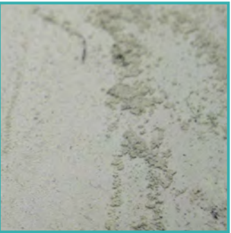
When scratched with a metal object, non-densified concrete wears and dusts easily. Densified and polished-concrete aid against erosion and wear, but cannot fully prevent it.
